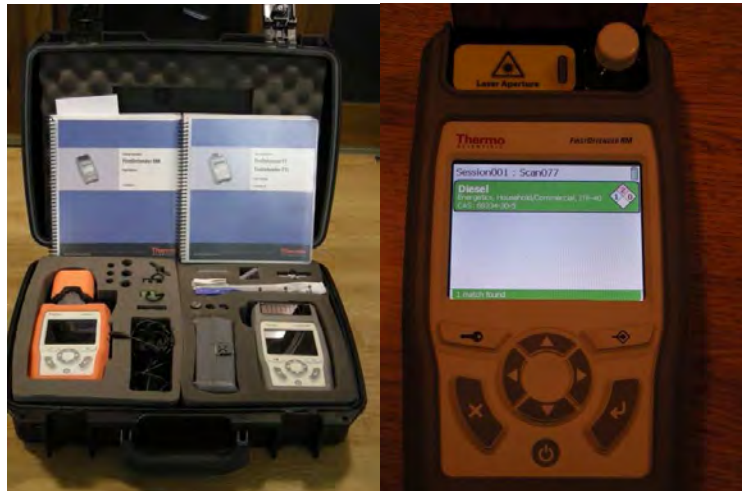
HazMat Team Chemical Identification Tools Image - On right is actual chemical identification screen from an incident sample.
